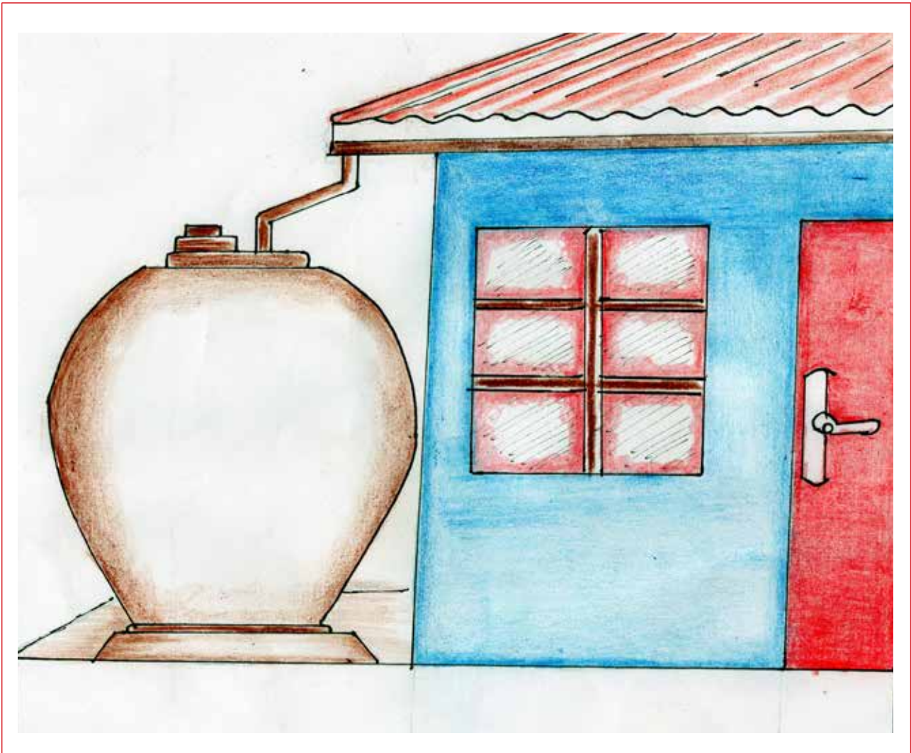
Figure 32: Hemispherical tank (Source: Uganda Landcare Network)
